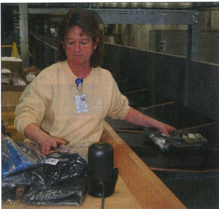
Items removed from the totes are scanned as they are placed on trays of the sortation system.
