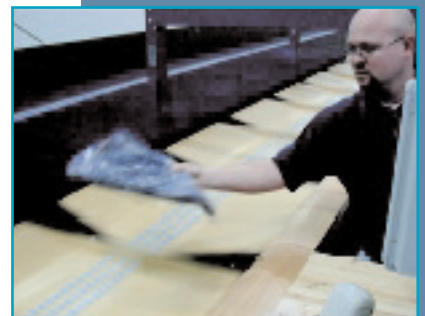
Softgoods items are manually scanned and placed on the tilt-tray sorter, then moved to the order packing stations.
