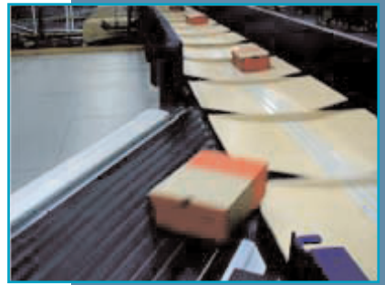
Footwear at Finish Line is picked to belts, then diverted onto the Erisplant tilt-tray sortation for delivery to the order packing stations.
