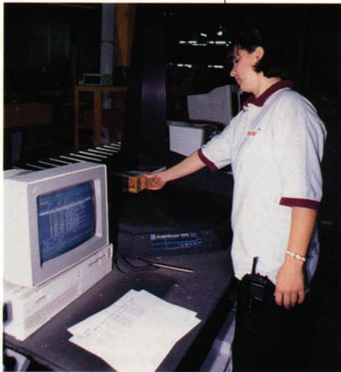
If a product's size and weight are not in the database, the item is placed in a cubing device to capture dimension information.
