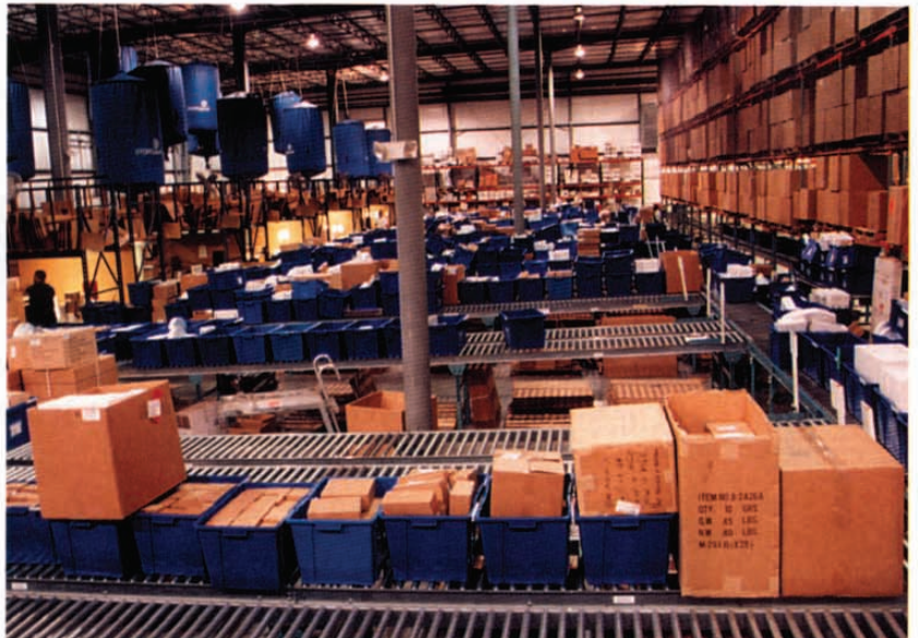
Ermanco technology amply covered Bakery Crafts' load requirements and provided non-contact accumulation to prevent product damage.
